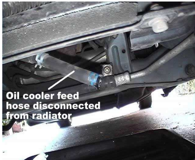
Fig 4. Disconnected Oil cooler feed hose
