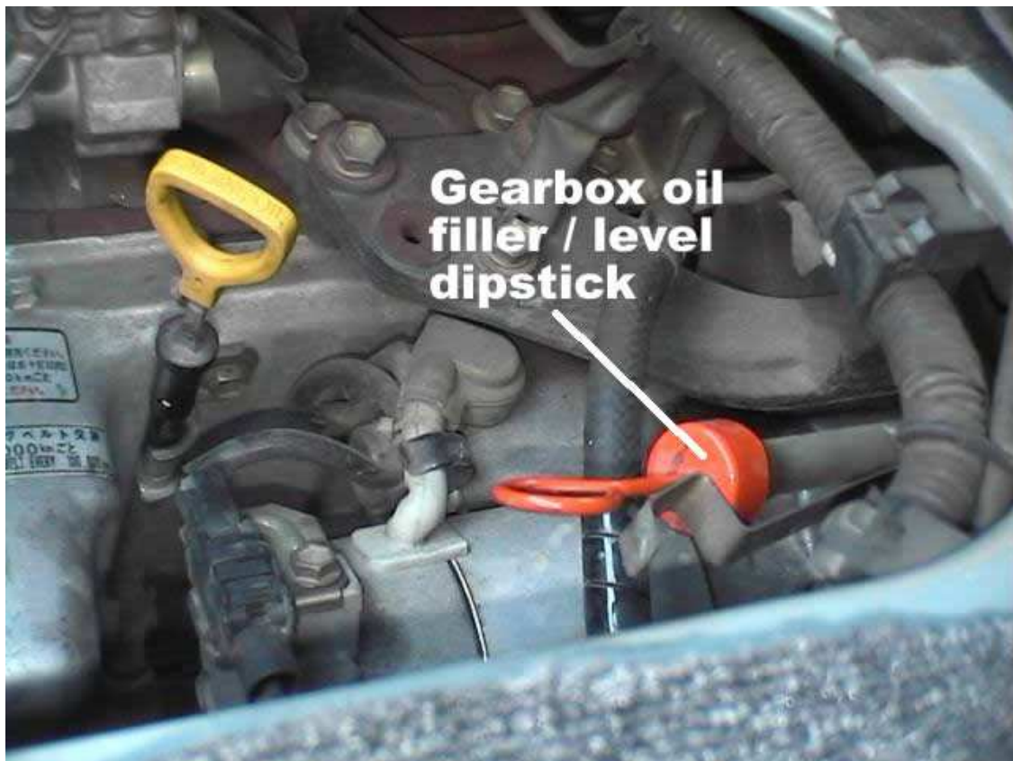
Fig1. Gearbox oil filler / level dipstick
